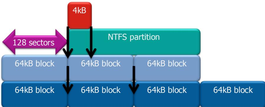
The same goes for a VMFS. When created through the ESX Service Console it will, by default, be misaligned. Use fdisk and expert mode to align the VMFS partition or create the partition through VMware vCenter which will perform the alignment automatically.
