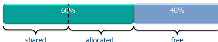
So when running Windows XP on ESX servers, if 60 percent of memory per client is actually being used, 50 percent of which is shared between clients, we need  $1 \text{ GB} \times 60\% \times 50\% = 300 \text{ MB}$  per client. Every VM needs about 5 percent more than the amount allocated as overhead from the host. So you need an additional 50 MB (5 percent of 1 GB) per client.
